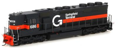
Since 2009, Athearn has provided the option of purchasing some of their models equipped with Tsunami sound. If you have an SD45 model without sound that you would like to upgrade, purchase SoundTraxx P.N. 885024. This board is designed to simply replace the factory PCB that supplies power to the locomotive. You can complete the installation in one to two hours with no modification required to the model!
