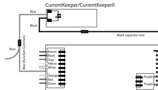
6. Solder the blue CurrentKeeper wire to the blue decoder wire and the black CurrentKeeper wire to the black decoder capacitor wire. Slide the pieces of heat-shrink tubing over the connections and heat to insulate. **Note:** Make sure you are soldering to the black capacitor wire remaining from Step 1, and not the black wire for rail pickups.
