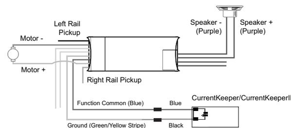
Connections for CurrentKeeper/CurrentKeeperII with TSU-1100 or ECO-100
